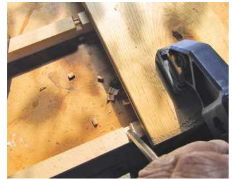
▲ Pic 3. A clamped-on fence helped to ensure that the notches for each shelf lined up accurately on the legs
